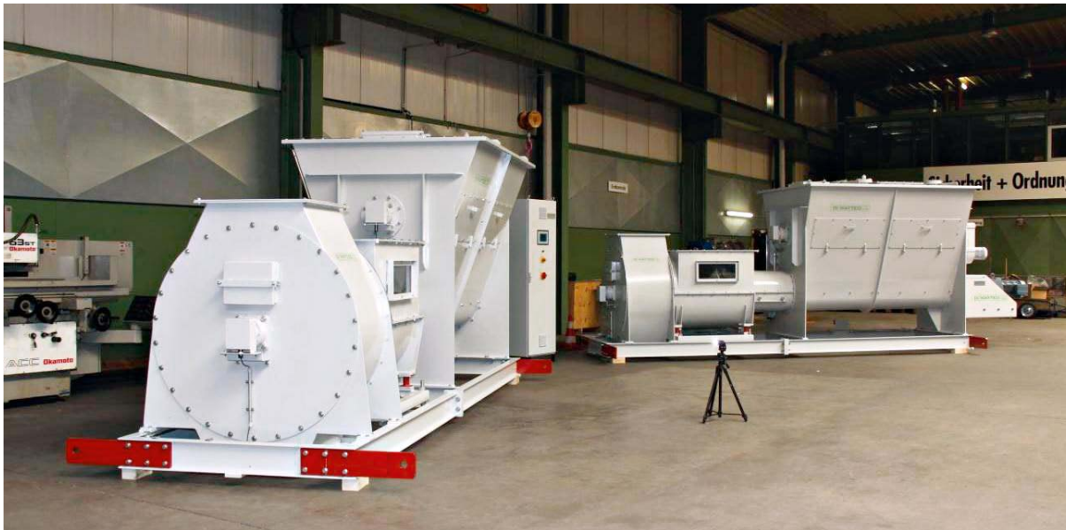
7 WeighTUBE® RWS tubular weigher for 15 tph in as-delivered condition
