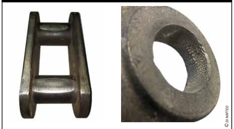
Figure 2: examples of a worn central chain of a bucket elevator
