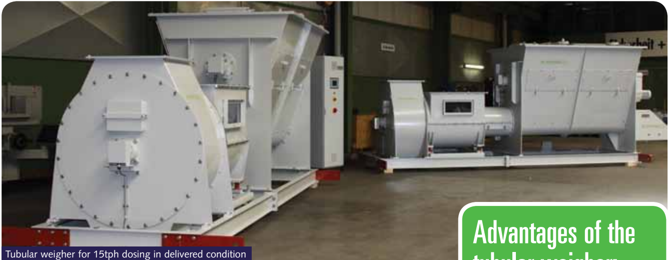
Tubular weigher for 15tph dosing in delivered condition
