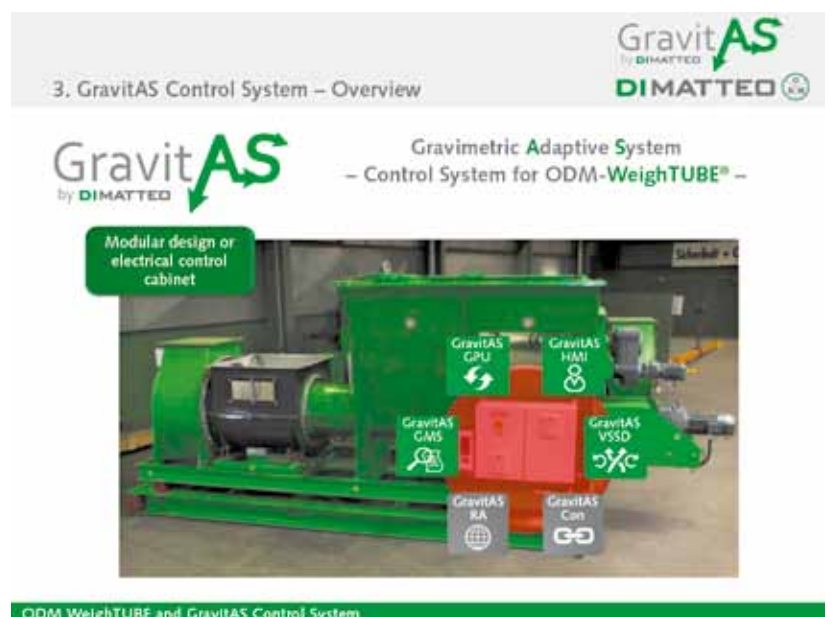
7 Fully assembled ODM-WeighTUBE® with GravitAS control cabinet
