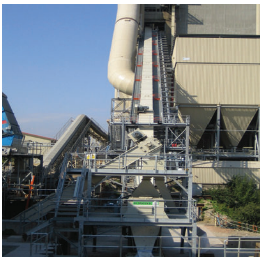
Fig.3 (left): Magnetic separator, ODM-DiscSCREEN and mechanical conveying by means of ODM-trough chain conveyor into the preheater-tower
